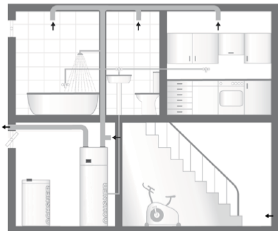
Exhaust system (single duct ventilation), exhaust air: from bathroom, WC, kitchen Air exit to outside free air
