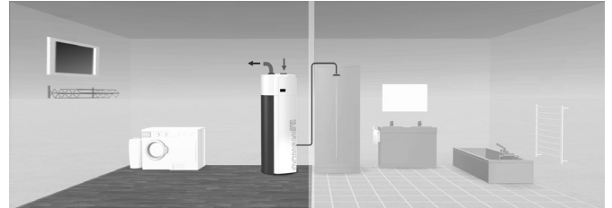
Installation in laundry room DHW heating from ambient air, drying of room
