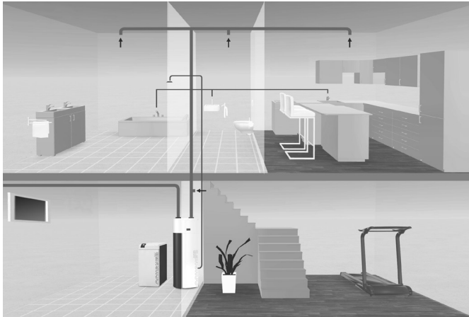
Exhaust air system (single-duct ventilation), Exhaust air from bathroom, WC and kitchen to outside
