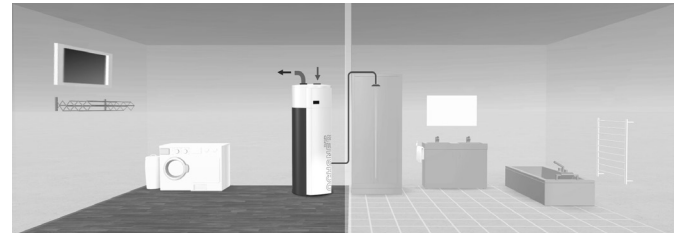
Installation in laundry room DHW heating from ambient air, drying of room
